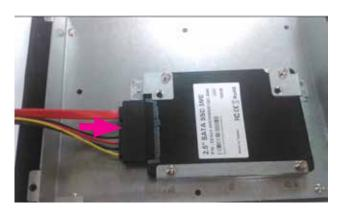
5. Make sure the SATA cable connectors (7-pin SATA signal and 4-pin SATA power connectors) are firmly plugged into the corresponding connectors on the motherboard.
