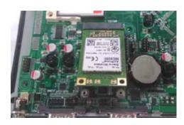
3. Press it down and lock the module with 2 screws.
