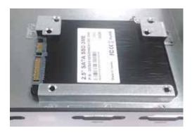
3. Lock the disk drive with 4 screws.
