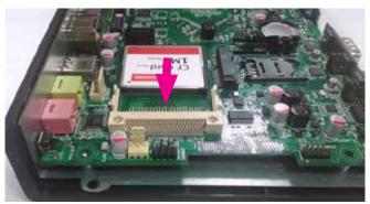
2. Press the card into the slot until it is firmly seated.
