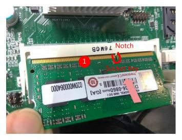
2. Press on both corners vertically until the module clicks into place.
