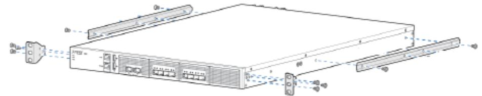
2. Slide the system into the rack, and secure the mounting ears to the rack, using two (2) rack-mounting screws on each side.
