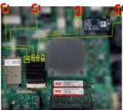
**2.** Align the notches of the module card with the socket keys in the slot. Tilt the end of gold fingers down while carefully inserting the card into the slot.
