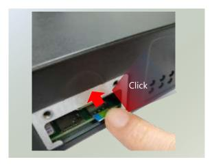
**3.** To remove the SIM card, use your fingertip to push it once and the card will automatically ejected.
