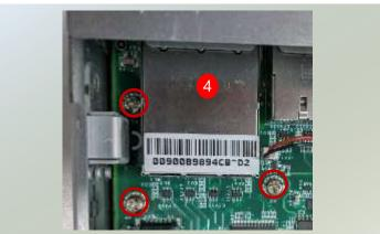
5. Replace the three (3) screws with the spacer standoff pillar studs.
