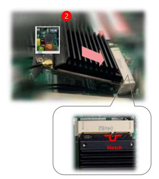
**3.** Secure the module with one (1) screw (included in the accessory pack).
