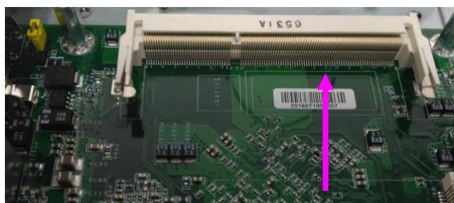
2. Align the DIMM module and make sure the notches of the module aligned with the socket keys in the slot.
