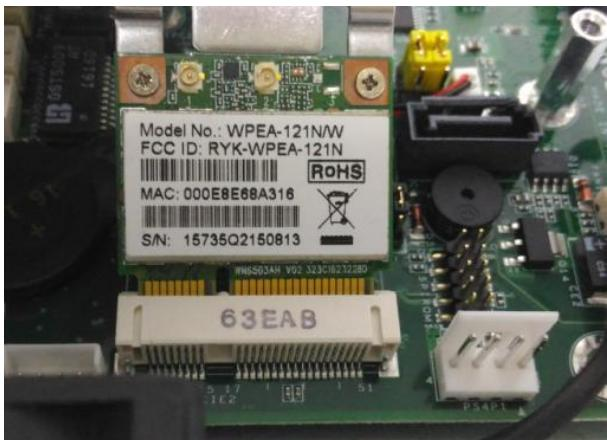
3. Press the module down and apply screws to secure it.
