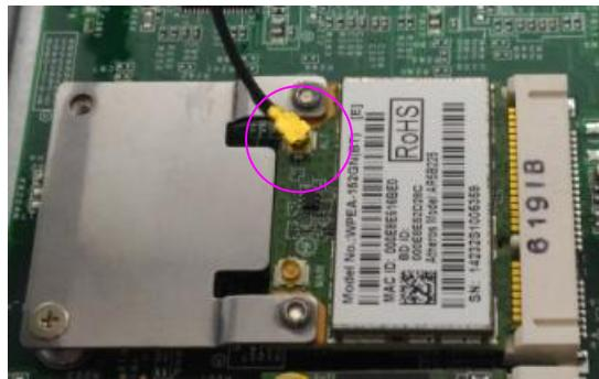
2. Plug the male connector of the SMA antenna onto the designated port as shown in the image below.
