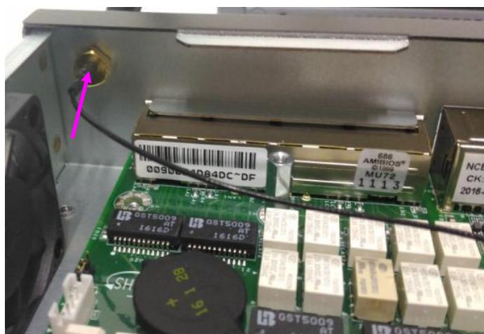
3. Use the supplied rings to secure the male connector from the front panel.
