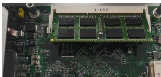
3. Insert the module into the slot at a diagonal angle and press it down until it's firmly seated by the clips at both sides.
