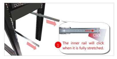
2. Hold the system with its front facing you, lift the chassis and gently engage the Rail Brackets on the model while aligning them with the slide-rail assemblies as shown in the image, and then push the system into the cabinet.
