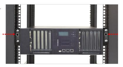
4. To remove the system from the rack, gently pull the system outwards towards you while pushing the Release Tab on both sides of the Rail Brackets.
