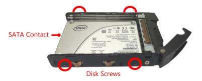
**2.** To install the mounted disk tray, push the tray into position in the chassis. Press on the hinge tab to close it.
