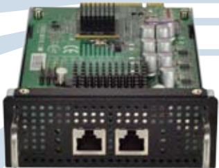
NCM-ITM201A: A 2-port Copper 10 GbE Module
