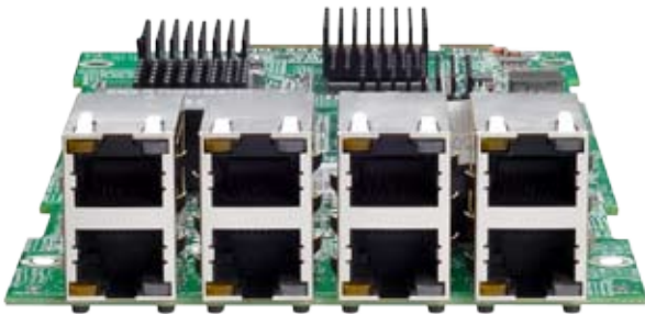
An 8 RJ-45 port NCM Module board
