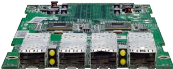
A 4 fiber port NCM Module board
