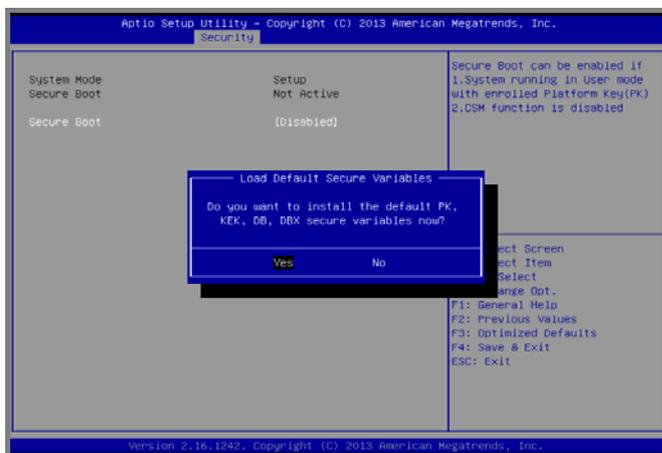
Once the status of Secure Boot is “active”, the system will be secured from being tampered by executions of unvalidated codes to attack your boot path or boot media.
