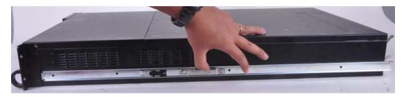
5. Securely attach the inner bracket to the side of the chassis by applying screws.
