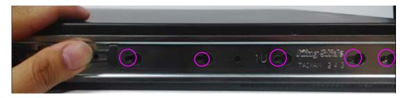
6. Lock the bracket onto the chassis with supplied screws. (Screws in different dimensions may not be able to securely attach the inner bracket).
