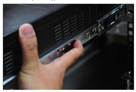
5. To bring the appliance out of the rack, use the two on the rail circled in the image below. When sliding the device out, remember to do it slowly.
