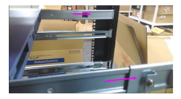
3. Gently push the model to the end of the rack to complete the installation. To slide
