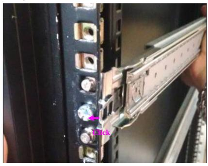
2. For the rear rack installation, also aim at 3 available holes and click the slide-rail assembly onto the rear rack.
