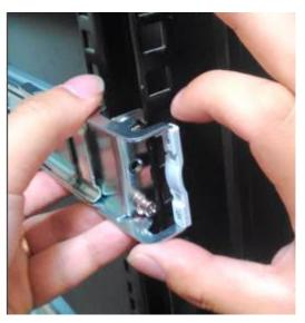
3. Repeat Step 1 and 2 for another slide-rail assembly in order to install in onto the rack.
