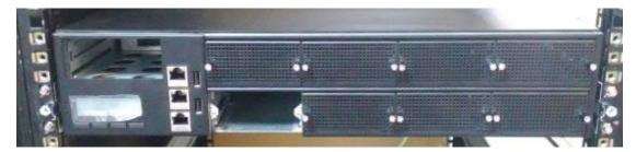
4. To slide the appliance out, gently pull it outwards. Then, press the slide-rail locks on both side and slide the appliance out.
