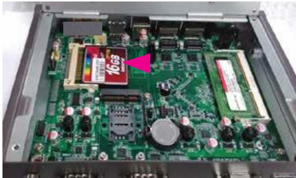
2. Press the card into the slot until it is firmly seated.
