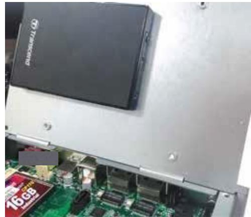
5. Connect the SATA cable as shown in the image below. First, plug the SATA connector of the cable to the disk drive, then place the 7-pin SATA signal connector and the 4-pin SATA power connector to the corresponding connectors on the motherboard.
