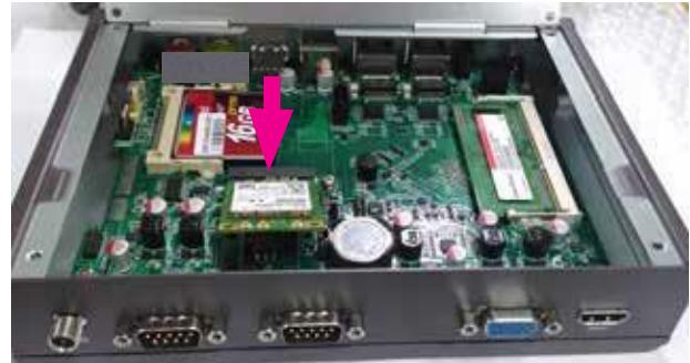
3. Press it down and lock the module with 2 screws.
