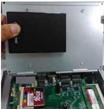
3. Lock the disk drive from the other side of the cover and apply four screws.
