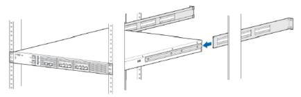
4. Secure the adjustable brackets to the rack, using two (2) rack-mounting screws on each side.
