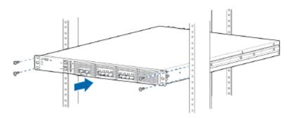
Note: Ensure the rear of the system is supported throughout the process of mounting the system into the rack.
