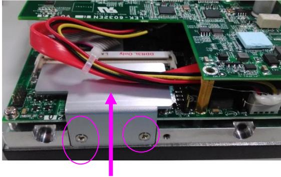
3. Align the memory module's key with the SO-DIMM socket's key.
