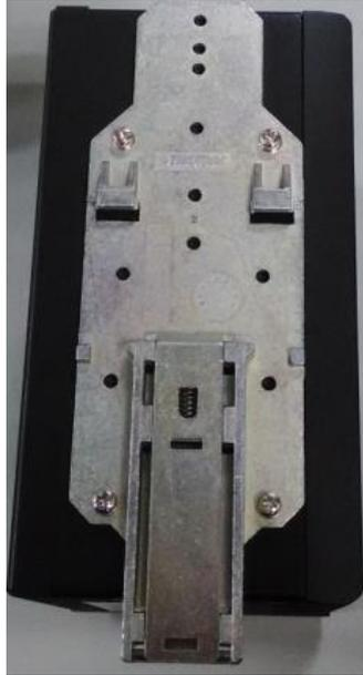
Hang the device onto a rail and push inwards until it firmly attaches.
