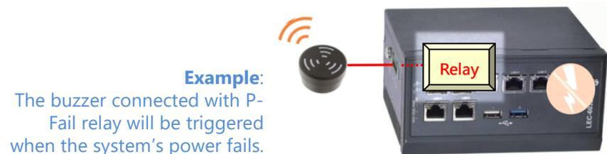
As LEC-6032C comes with dual power and P-fail relay features, the P-Fail relay will have the signaling device triggered as the power supply fails. LEC-6032C's relay circuit is set to be **Open** by default and **Closed** when either or neither of the powers is detected; the **Closed** (or **Short**) circuit then allows the Alarm Device to be activated.
