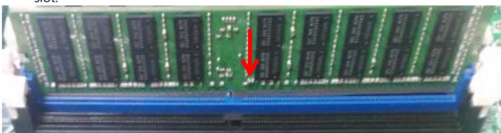
4. Insert the module into the slot until it's firmly seated and close the latches.
