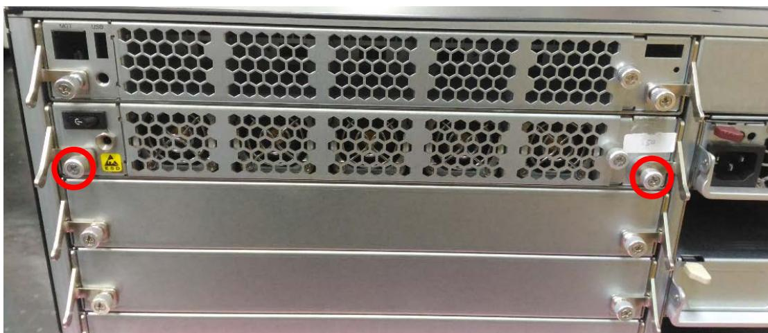
3. Hold onto both captive screws and handles and lift them upwards at the same time.
