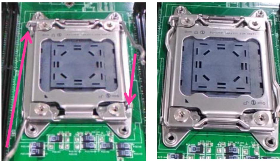
7. Put the heat sink on the installed CPU and match the screws with the screw holes on the board. Fasten two screws which are opposite to each other at a time and then the other two. It is easier this way to avoid the force of spring.
