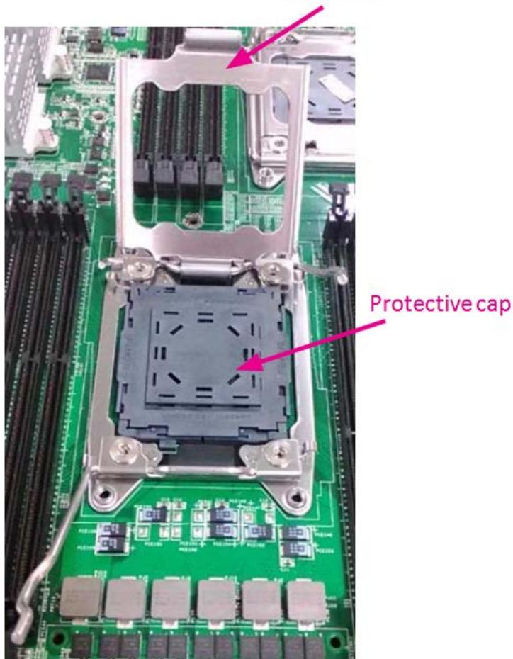
5. Align the CPU and the notch on the socket. The CPU should fit perfectly into the socket. Note that the CPU fits in the socket in only one direction.
