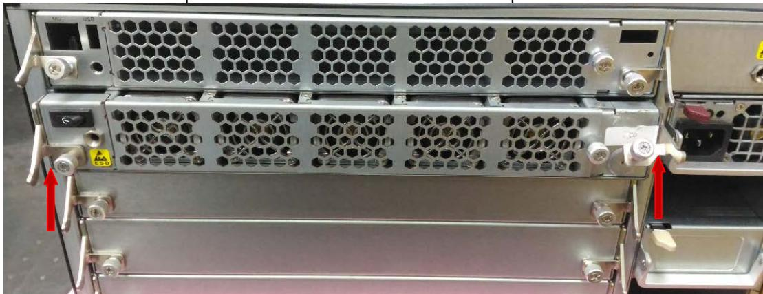
4. Apply some force to pull the CPU blade out.
