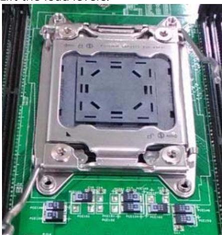
4. Open the load plate and also the protective cap.
