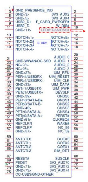
**Pin 10** is connetectd with **Pin 42** on Mini-PCIe through a zero-ohm resistor for LED indicator.
