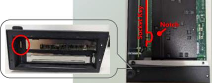
4. Gently insert the module pins into the socket until it is fully seated.
