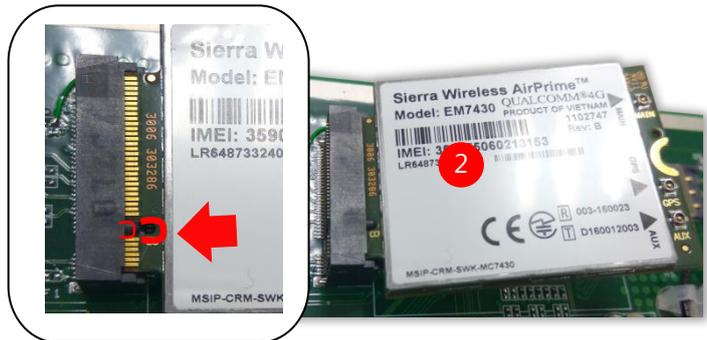
3. Push down on the module and secure it with the screw that comes with the package.
