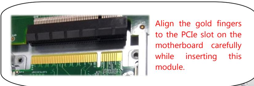
Align the gold fingers to the PCIe slot on the motherboard carefully while inserting this module.
