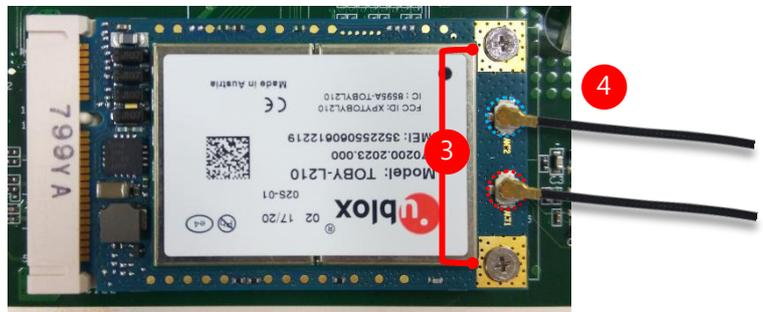
4. Snap one LTE antenna cable onto the U.FL connector for **Main**, and the other one onto the U.FL connector for **AUX**.
