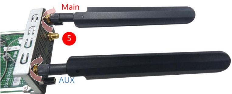
5. Attach the LTE antennas onto the front panel. Make sure the connector for **Main** and the connector for **Aux** are connected to the front panel as shown in the picture.
