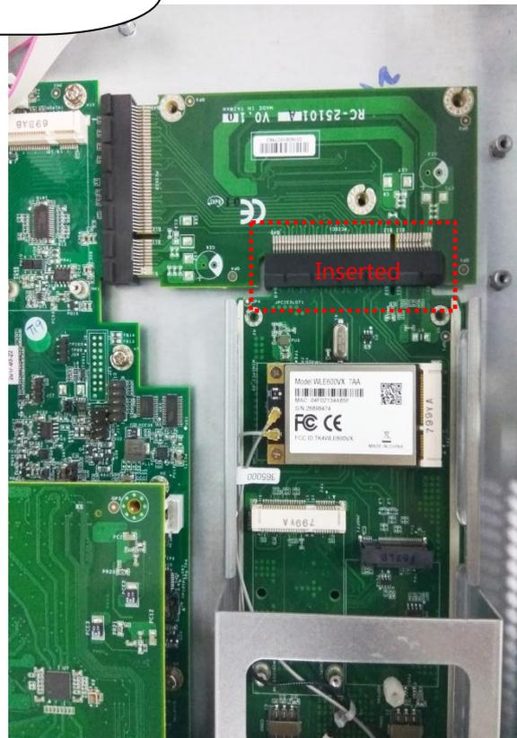
4. Once the expansion card is firmly seated, rotate clockwise and tighten the two lock-screws to secure the card, and then recover the system's top cover.
