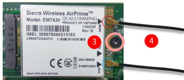
4. Snap one LTE antenna cable onto the U.FL connector for **Main**, and the other one onto the U.FL connector for **AUX**.
