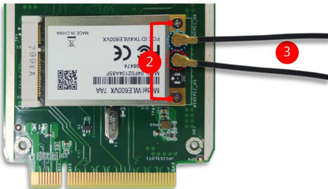
4. Attach the Wi-Fi antennas onto the front panel. Make sure the connector for **WIFIO** and the connector for **WIFI1** are connected to the front panel as shown in the picture.
