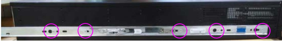
6. Repeat Steps 1 to 5 for another slide-rail and attach its inner bracket onto another side of the chassis.
