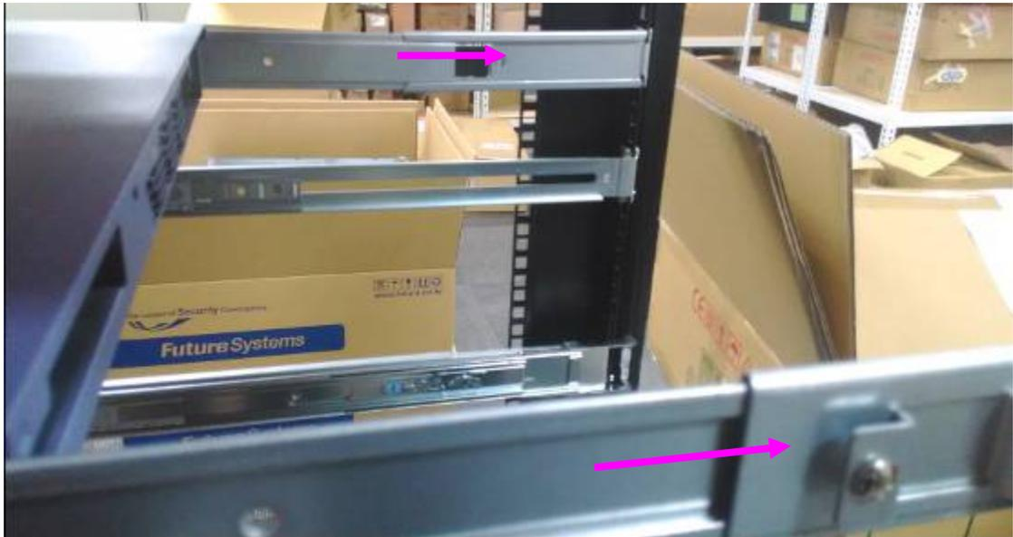
3. Gently push the model to the end of the rack to complete the installation. To slide
