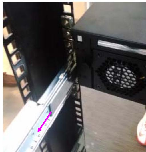
2. Simultaneously push the release tabs on both sides in the arrow of direction below, while pushing the appliance into the end of the rack.
