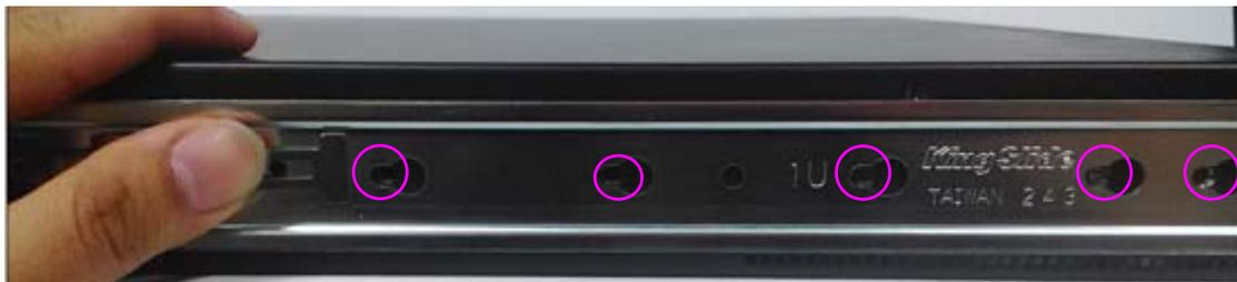
6. Lock the bracket onto the chassis with supplied screws. (Screws in different dimensions may not be able to securely attach the inner bracket).
