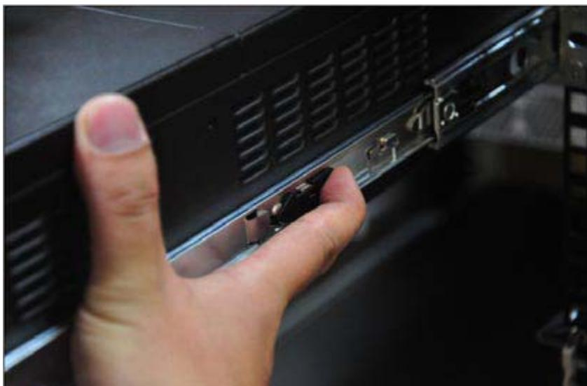
5. To bring the appliance out of the rack, use the two on the rail circled in the image below.
