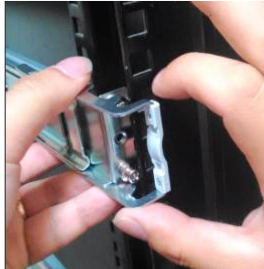
3. Repeat Step 1 and 2 for another slide-rail assembly in order to install in onto the rack.
