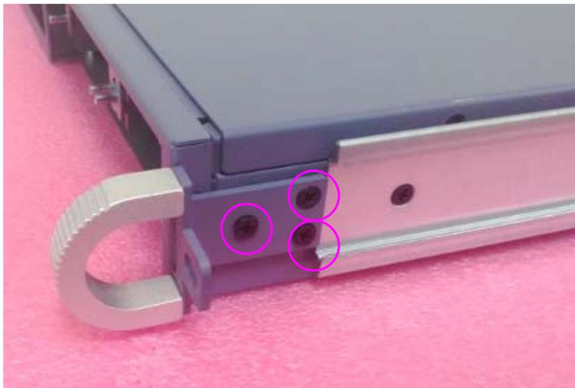
6. Repeat Step 4 and 5 for another ear bracket set to attach to the front of the chassis
