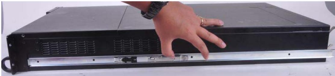
5. Securely attach the inner bracket to the side of the chassis by applying screws.
