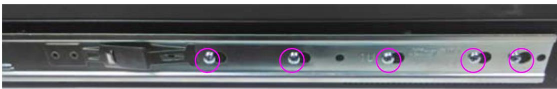
7. Do the same with another inner bracket to attach the rest of the area of the same side chassis.
