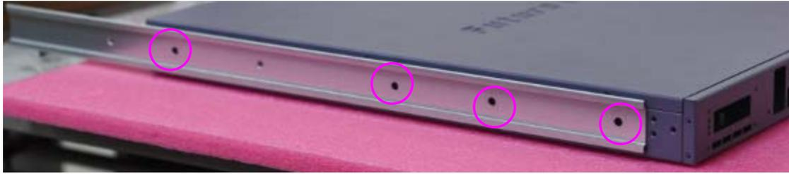
3. Repeat Step 1 and 2 for another inner bracket to attach on the other side of the chassis.
