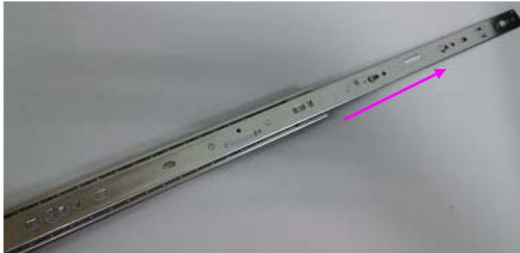
3. Push the white slide-rail lock outwards as the arrow of direction below. Then pull the inner bracket out of the slide-rail assembly.
