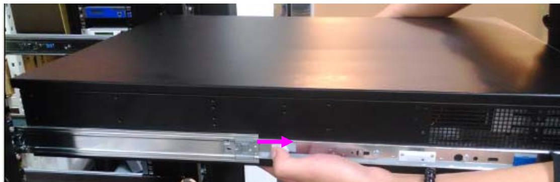
Notes: the process of sliding-in and sliding-out should be smooth. If not, please adjust the mounting tips.
