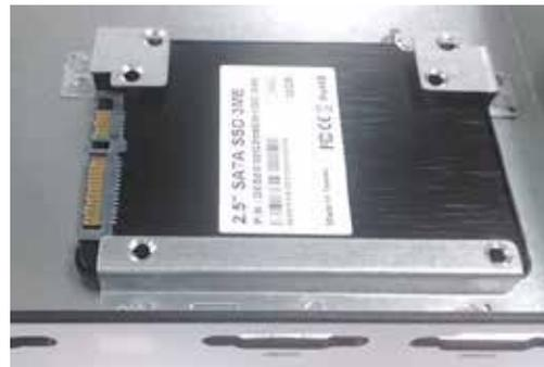
3. Lock the disk drive with 4 screws.
