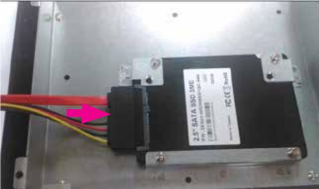
5. Make sure the SATA cable connectors (7-pin SATA signal and 4-pin SATA power connectors) are firmly plugged into the corresponding connectors on the motherboard.
