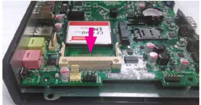
2. Press the card into the slot until it is firmly seated.
