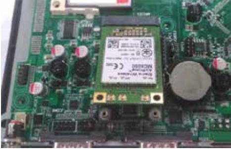
3. Press it down and lock the module with 2 screws.
