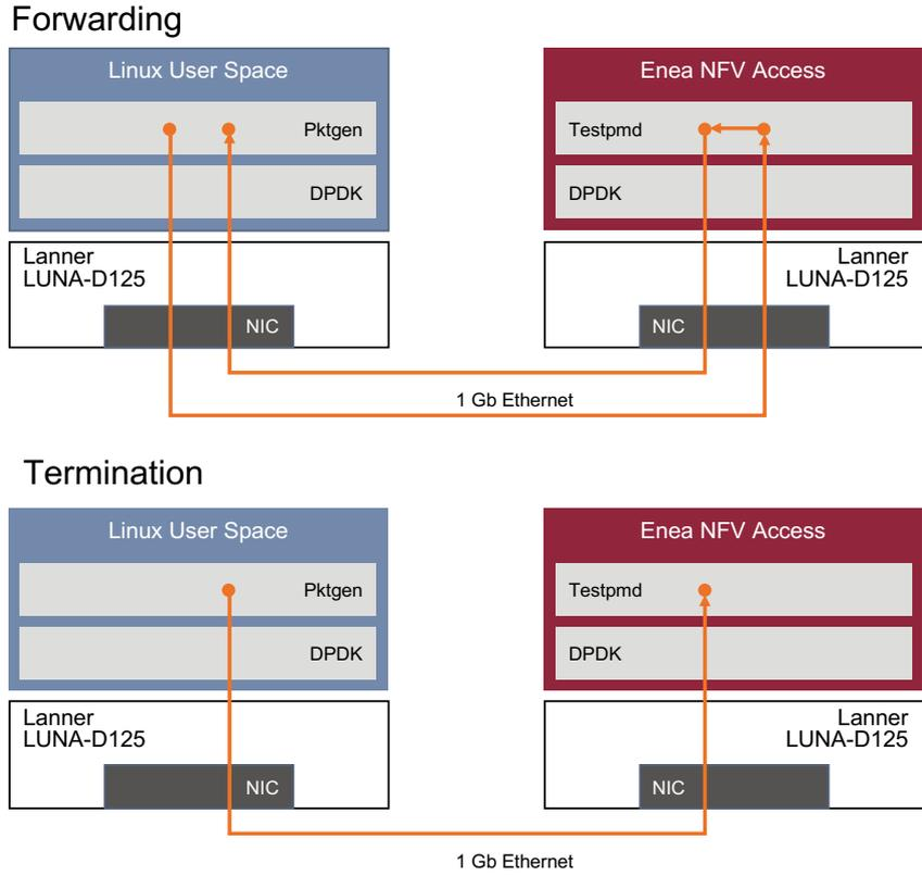
Figure 2. Test configurations for traffic forwarding test (top) and traffic termination test (bottom).<sup>4</sup>
