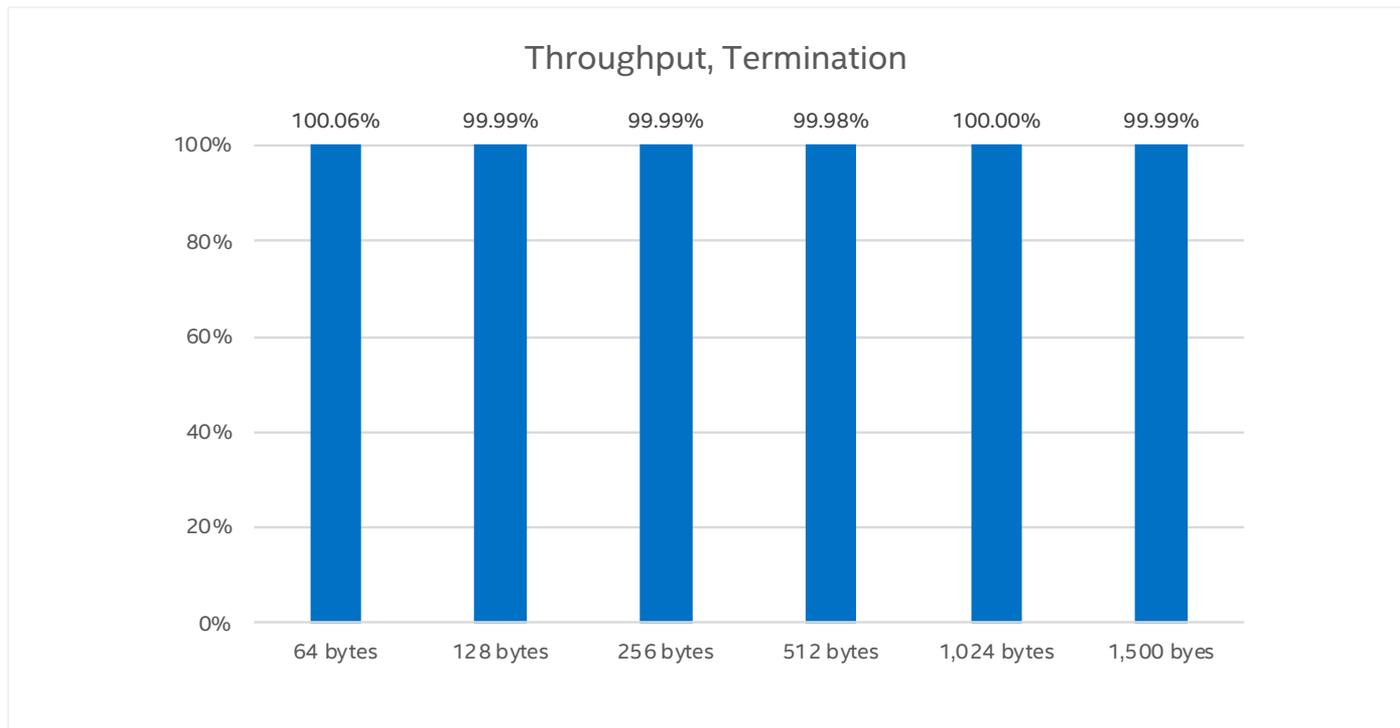
Figure 4. Termination results from tests on LUNA-D125 with Enea NFV Access.<sup>3</sup>
