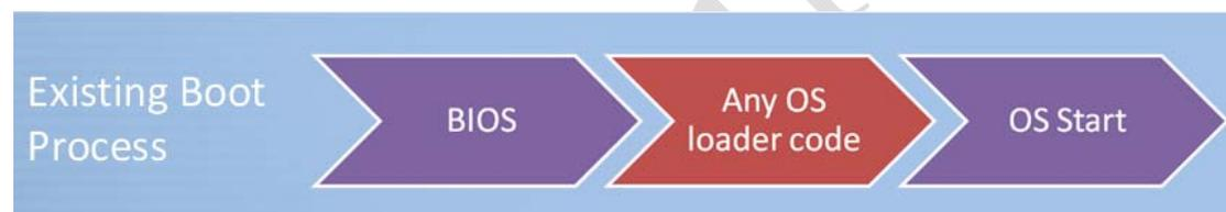
In the "Secure Boot Process", the UEFI BIOS will only launch a verified OS boot loader. Malware cannot replace the boot loader.
