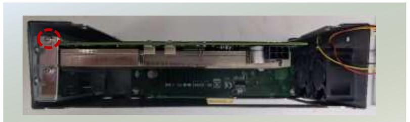
6. The module installation is complete. Make sure to cover the system with the chassis and secure in place with screws.
