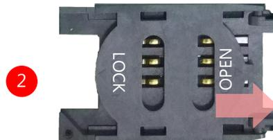
3. Insert the SIM card into the slot in the cover with the gold contacts facing down, and the angled corner of the card is positioned correctly as shown in the picture.
