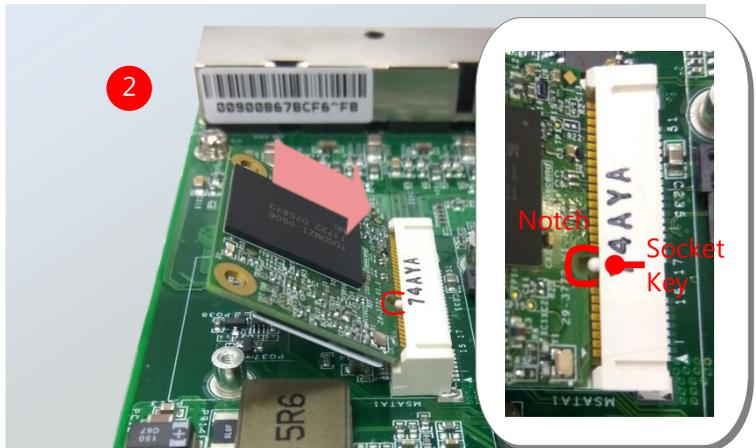
3. Push down on the module and secure it with the screw that comes with it.
