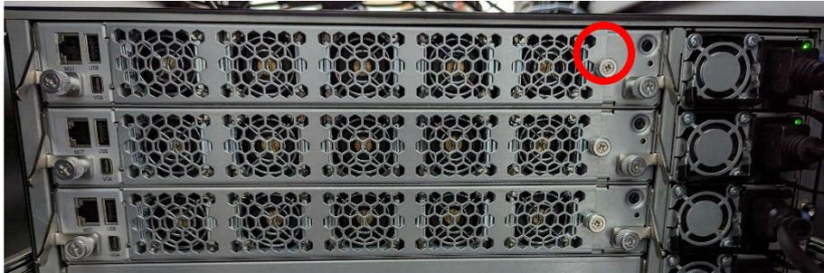
3. Hold onto the loosened captive screw and remove the bezel.
