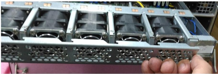
4. Take the worn-out fan out of its original place, and insert a new fan into the system. Repeat same steps for additional worn-out fan.
