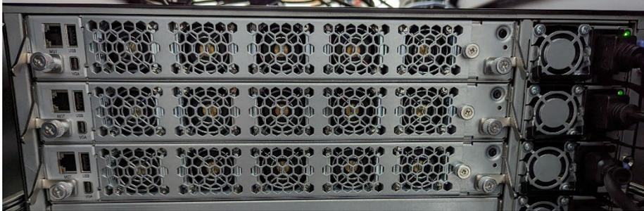
2. Rotate and loosen the captive screws circled in the image below. You may apply a screwdriver to conduct this task.
