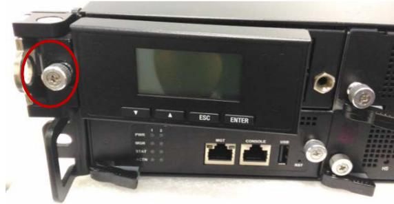
2. Open the hinge LCM and locate the HDD/SSD bays as the images shown below.
