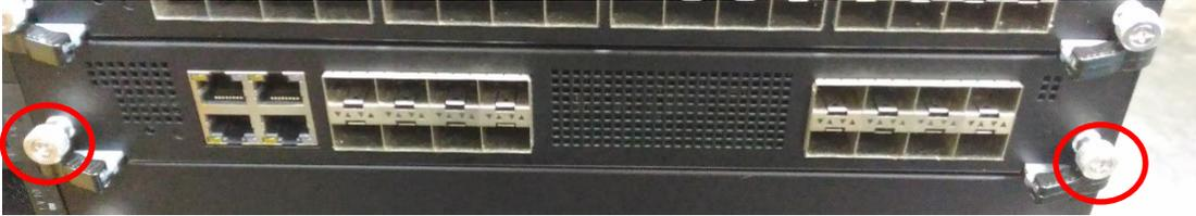
2. Pull the two lock-handles frontwards, then extend outwards.
