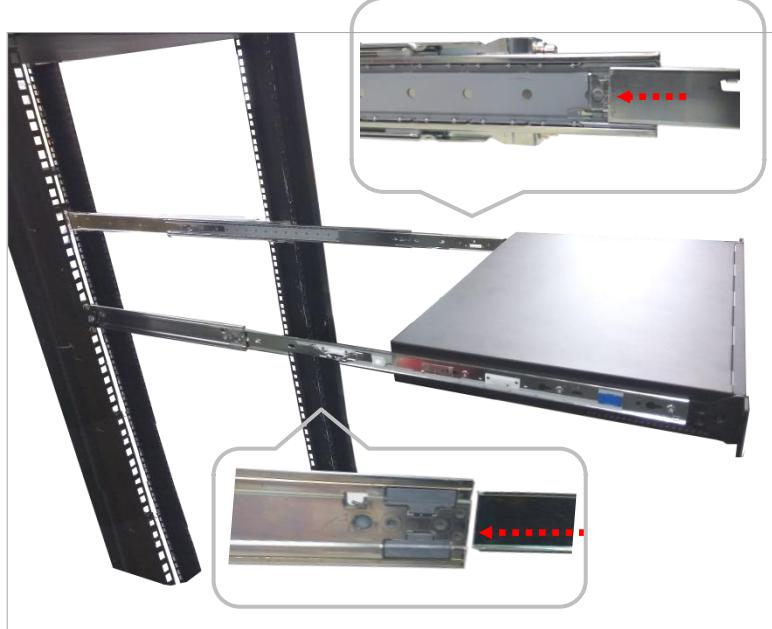
3. Keep sliding the rails in until they stop about halfway. Press down on the metal clips on both Inner Channels and push them further into the rack cabinet.
