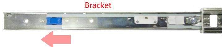
3. Locate and push the Release Tab on the bracket to detach the bracket from the Inner Channel, and carefully slide it out.
