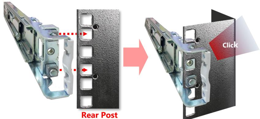
2. Repeat Step 1~2 to install the other rail onto the rack post.
