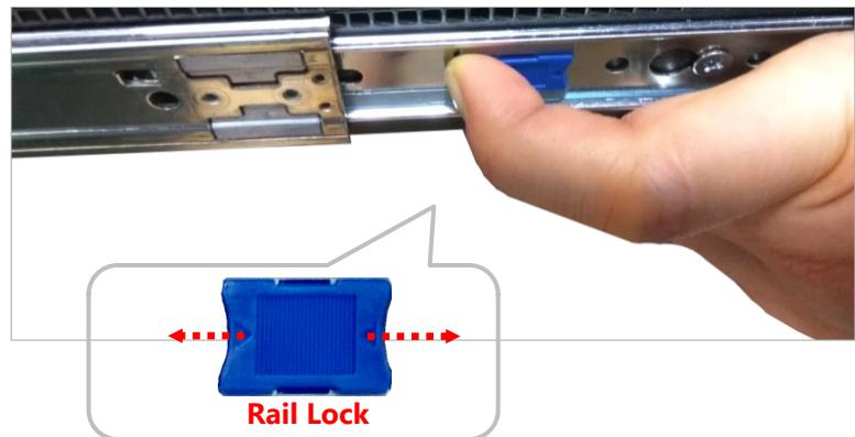
4. Push the system all the way in until the rack. The installation is complete.
