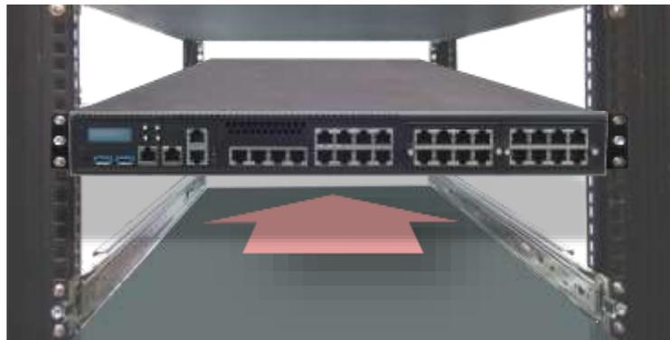
To detach the chassis from the rack, pull the Release Tabs on both sides of the brackets towards you while gently sliding the chassis out.
