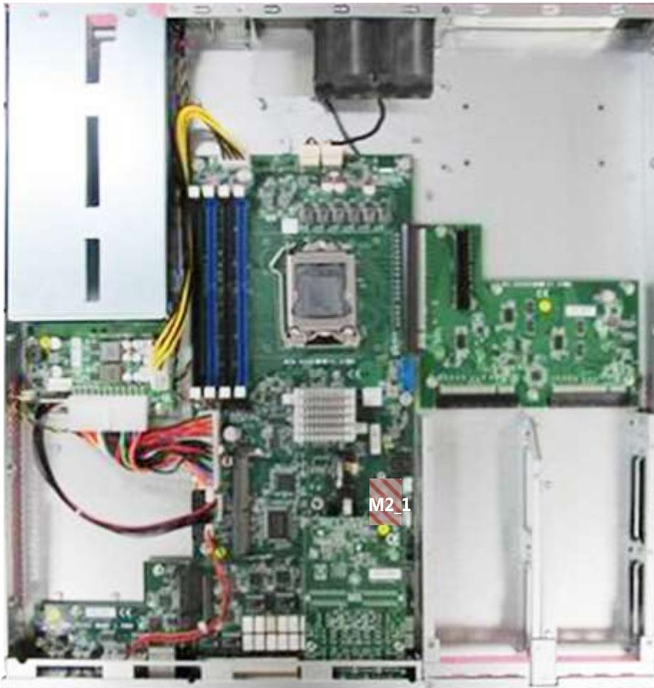
2. Insert the M.2 module into the slot at 15° angle, align the notch on the module with the corresponding socket key in the slot, and then secure it with a screw.
