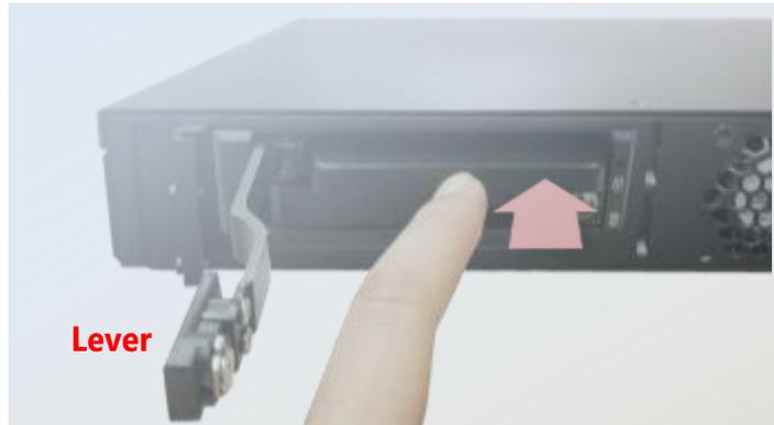
Push the lever back to close the slot; the mechanism of the caddy will have the SSD connected into the socket automatically.
