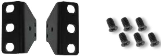
Take an ear bracket, align the holes on it with those on the side of the system, and lock it onto the system with three provided screws. Do the same to the other ear bracket.
