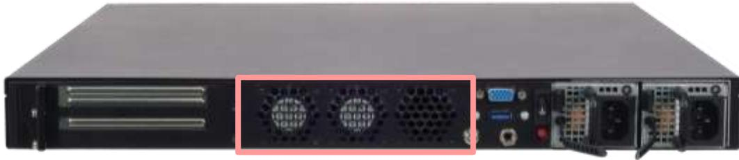
1. From the rear side of the fan, loosen the screw that secures the fan connector.
