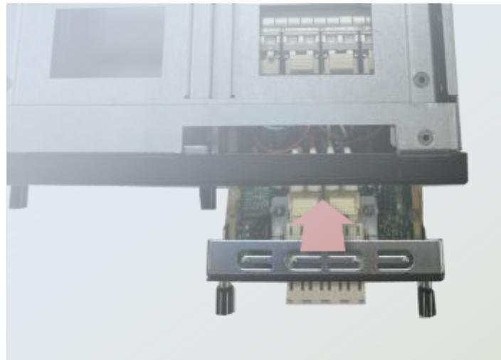
4. Once the module is firmly seated, rotate clockwise and tighten the two lock-screws.
