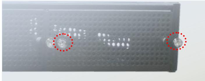
3. Insert your NIC Ethernet module. (The module shown in the image below is for reference only)
