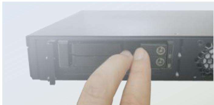
7. Lock the tray with the provided key. Turn the key 90° clockwise to the "Locked" position.
