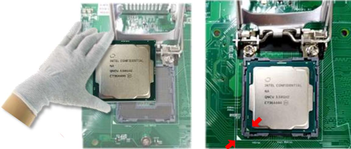
4. After the processor is correctly seated in the socket, lower the lever along with the plate, slide the end of the lever into the locking position.
