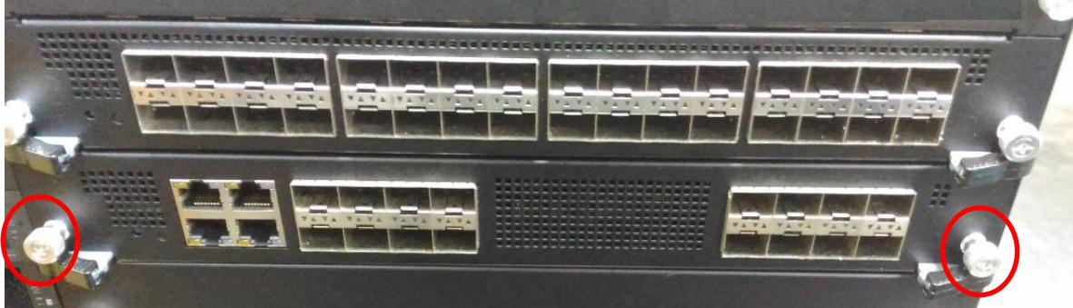
2. Pull the two locks towards the directions as shown in the arrows of directions below.
