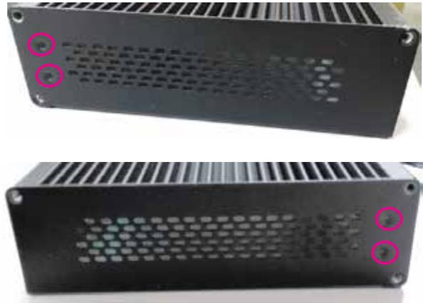
3. Attach the L-shaped brackets to the screw holes on each side of the system, as the image below. Apply screws to secure the brackets until totally fixed.
