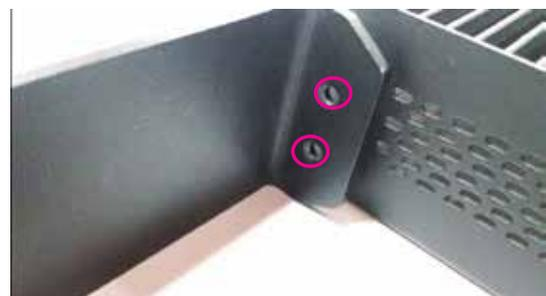
4. Attach the ears of the L-shaped brackets to the rack and then apply long threaded nails.
