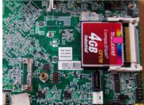
3. Apply a supplied screw to secure the CF card.
