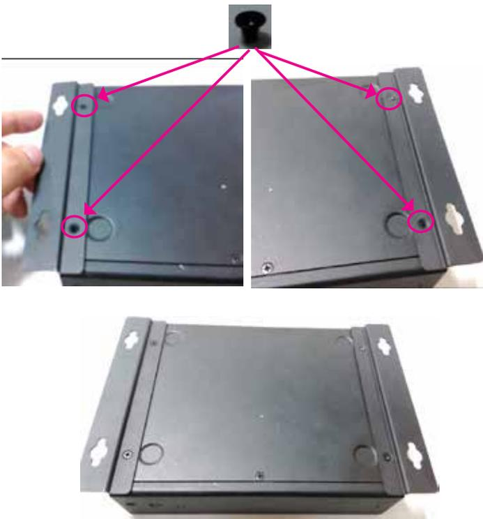
4. Place the system on where it will be mounted on the wall.
