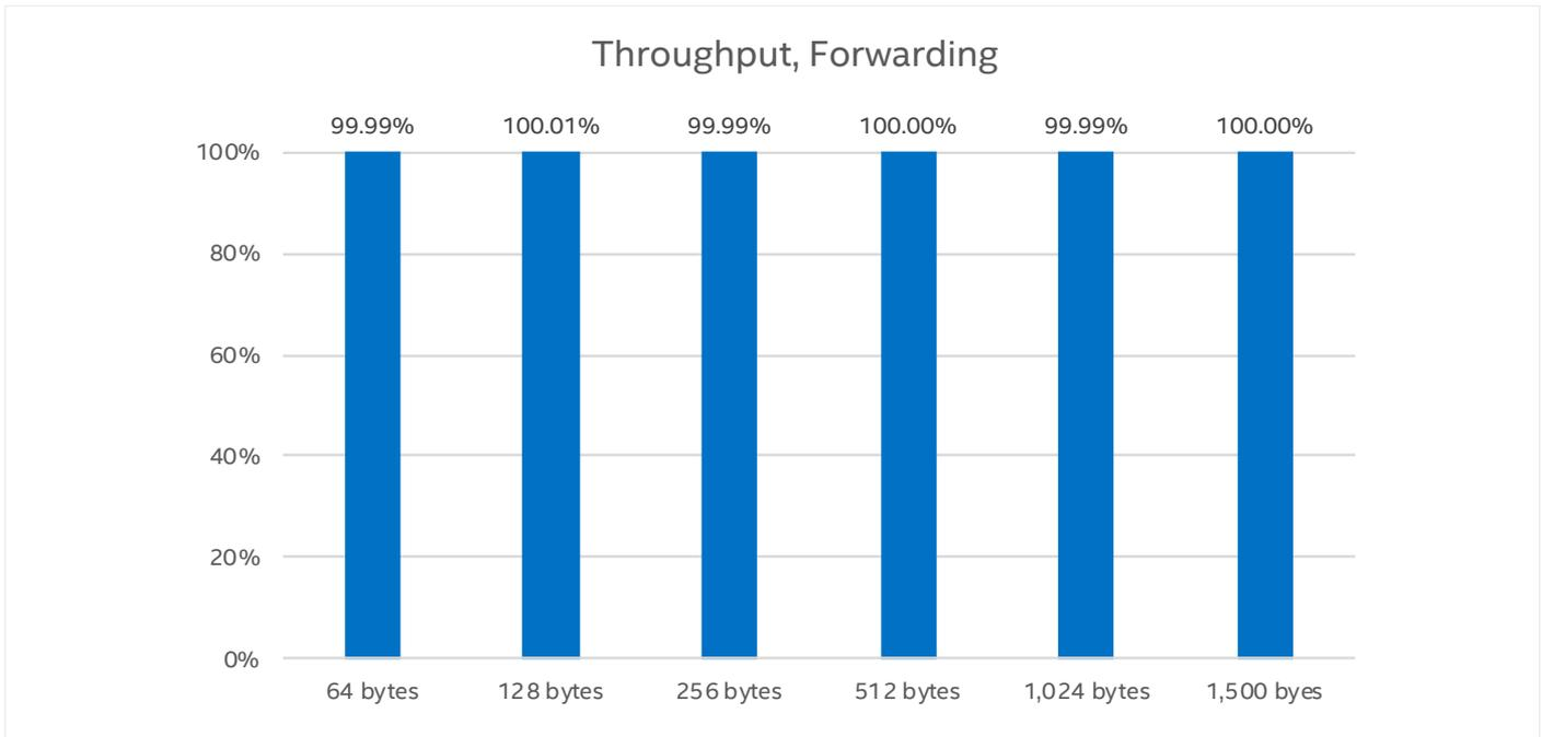
Figure 3. Throughput results from tests on LUNA-D125 with Enea NFV Access.<sup>3</sup>
