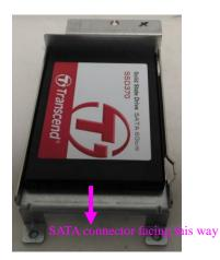
4. Turn the tray with SSD upside down and apply four screws.
