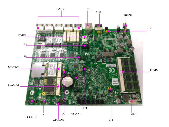
Notes: the DIMM and mini-PCIe modules shown as installed in the picture are for reference ONLY and NOT included by default.
