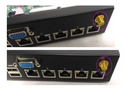
4. Tighten the rings and install the antenna. When installing the antenna, rotate it until it is tightened.
