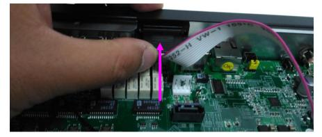
3. Align the DB15 connector as shown in the image below. Then apply its two original bolt screws to fix it.
