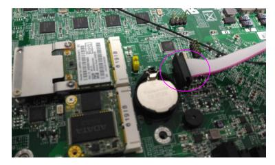
2. Place the DB15 VGA connector at its approximate location on the front panel.
