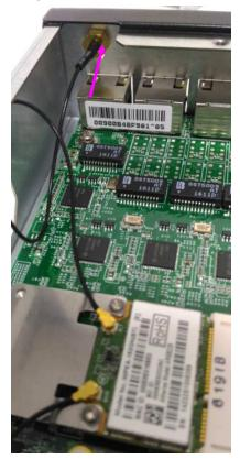
3. Use the supplied rings to secure the male connector from the front panel.
