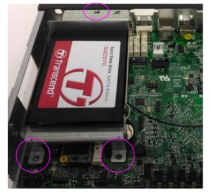
6. Connect the SATA 7-pin signal cable and the SATA 4-pin power cable to their corresponding connectors on the motherboard.
