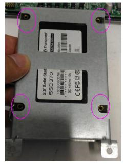
5. Place the SSD-installed tray back onto the system. Apply three screws back.
