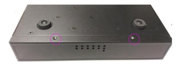
3. Slide the compartment as the arrows of directions below to access the inside of the system.
